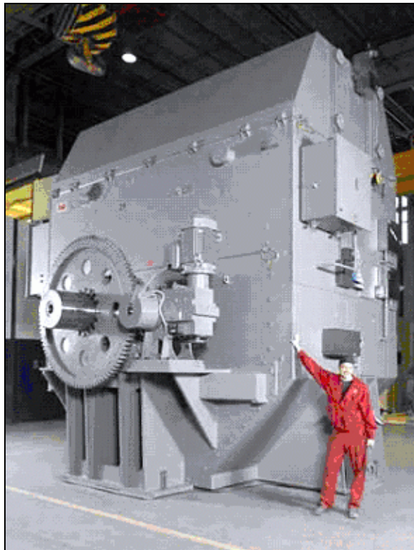
Figure 3.21: A compressor motor with a rated output of 24 MW [95, Savolainen, 2005]
