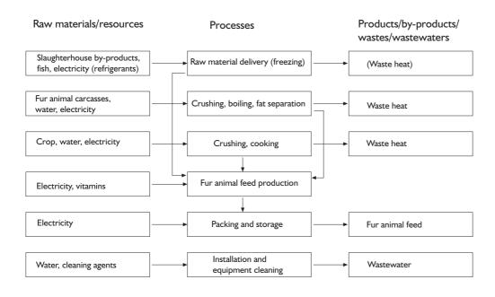
Figure 6. A typical flow scheme of fur animal feed production.
