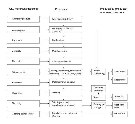
Figure 5. A typical flow scheme of rendering.
