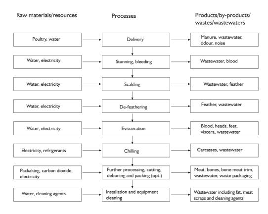
Figure 4. A typical flow scheme of poultry slaughtering.
