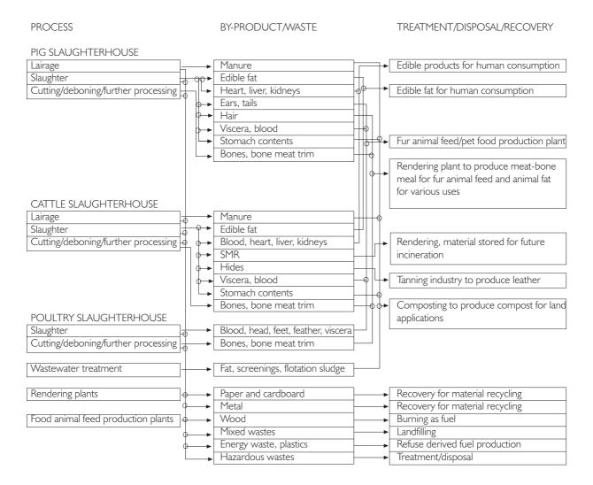
Figure 10. Current recovery and disposal of solid by-products and wastes produced in the Finnish slaughterhouses, rendering plants and fur animal feed production plants.
