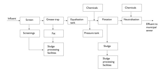
Figure 7. A typical flow scheme of slaughterhouse wastewater pre-treatment.
