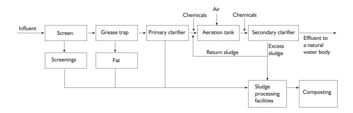
Figure 8. A flow scheme of the wastewater pre-treatment of a fur animal feed production plant discharging its wastewater into a natural water body.
