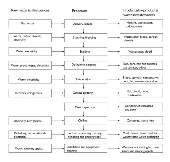
Figure 2. A typical flow scheme of pig slaughtering.
