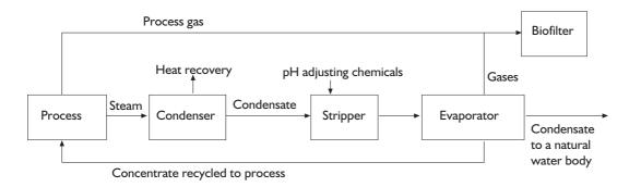
Figure 9. The flow scheme of a rendering plant wastewater treatment process.
