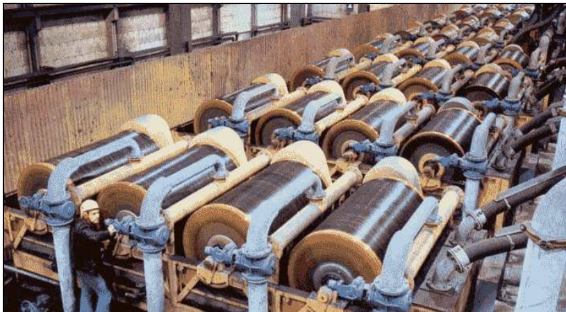
Figure 2.17: Low-intensity drum separators
