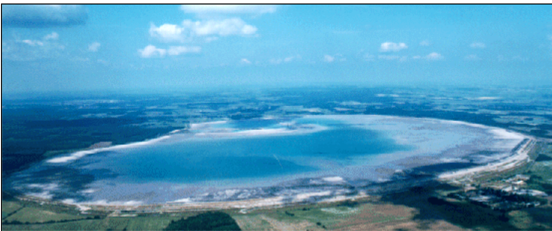
Figure 1.23: Example of a large tailings pond (330 Mm 3 )
