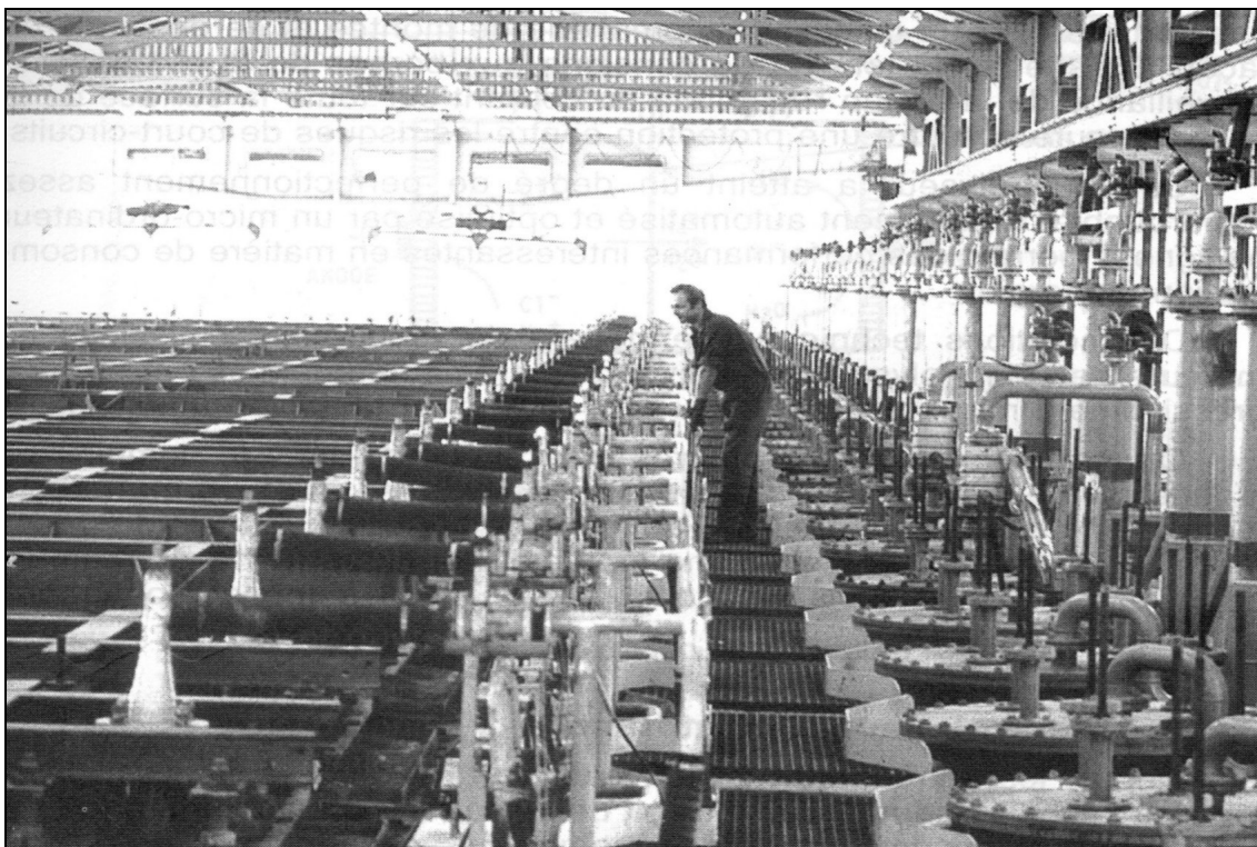
Figure 2.5: Mercury cells with vertical decomposer [Le Chlore, 1996]
