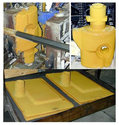
Figure 2.33: Croning cores (top) and moulds (bottom) [237, HUT, 2003]
