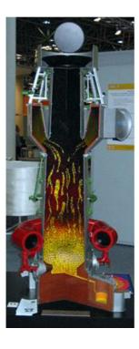
Figure 2.9: Schematic outline and miniature model of a (cold blast) cupola furnace [44, ETSU, 1993], [237, HUT, 2003]
