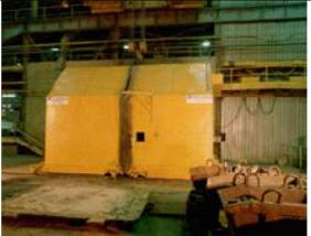
Figure 4.17: Doghouse cover for a shake-out grate, for large-size batch castings [209, Metalodlew s.a., 2003]
