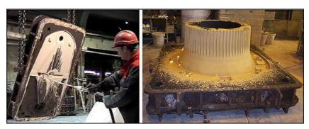
Figure 2.34: Flow coating with alcohol-based coating, followed by firing or drying [237, HUT, 2003]
