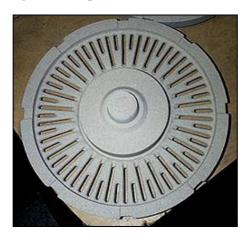
Figure 2.32: Cold-box core [237, HUT, 2003]
