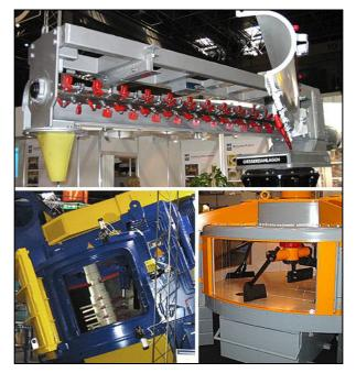
Figure 2.29: Various types of sand mixers [237, HUT, 2003]
