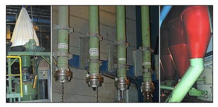
Figure 2.8: Pneumatic conveyors and silos for powdered materials [237, HUT, 2003]
