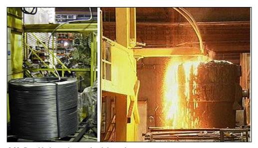
Figure 2.22: Deoxidation, using an aluminium wire [237, HUT, 2003]
