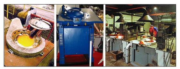
Figure 2.14: Coreless induction furnaces [237, HUT, 2003]
