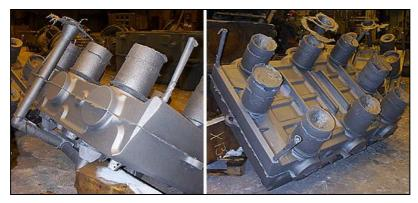
Figure 2.49: Casting with running and gating system [237, HUT, 2003]
