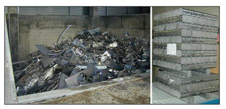
Figure 2.7: Aluminium scrap(l.) and ingots (r.) [237, HUT, 2003]
