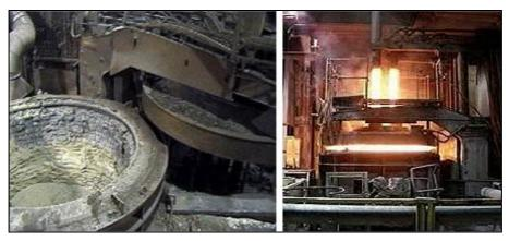
Figure 2.12: EAF furnace [237, HUT, 2003]
