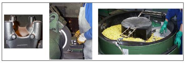
Figure 2.51: Burrs (l.) and their removal using a grinding stone (m.) and slide grinding (r.) [237, HUT, 2003]
