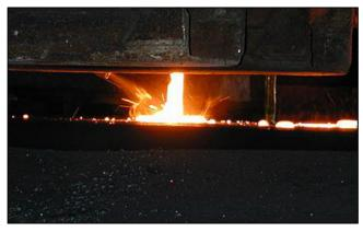
Figure 2.24: Inoculation during pouring [237, HUT, 2003]
