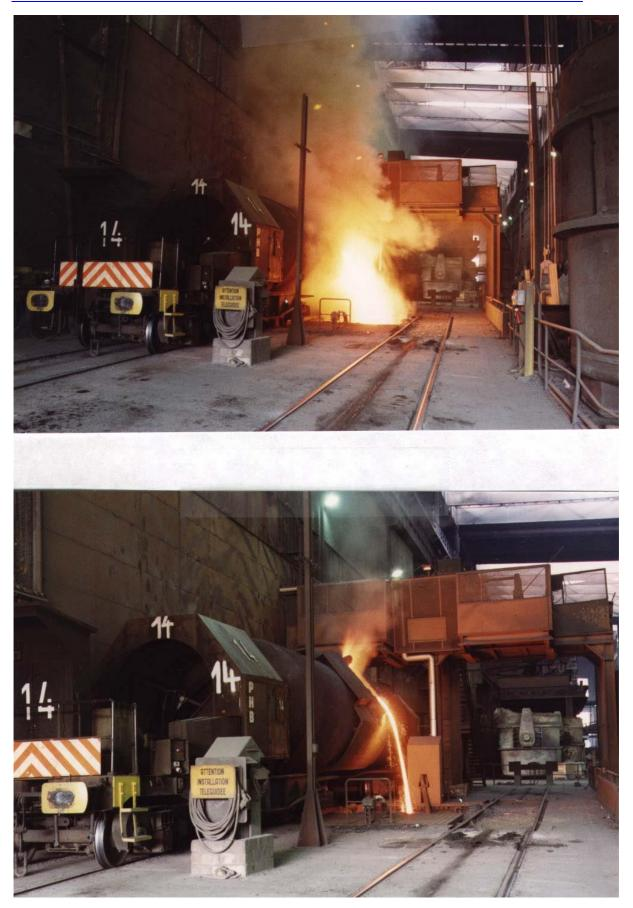
Figure 8.21: Reladling of hot metal from torpedo ladle to charging ladle with and without dust/fume suppression with inert gas (CO<sub>2</sub>) [UNEP, 1997]
