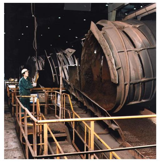
Figure 5.1 : Balling drum as part of a pelletisation plant
