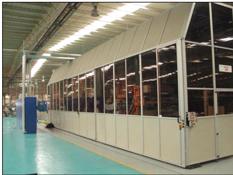
Figure 4.2 Encapsulated integrated chromium plating line [140, Atotech, 2003]
