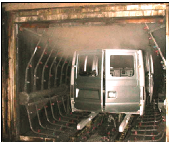
Figure 2.4: Automotive body undergoing spray pre-treatment [ACEA]
